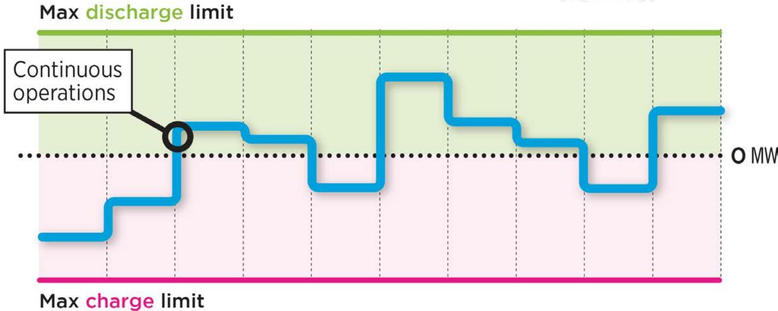
Continuous operation mode - ESRs can update their max charge and discharge limits hourly in day-ahead and more frequently in real-time.
