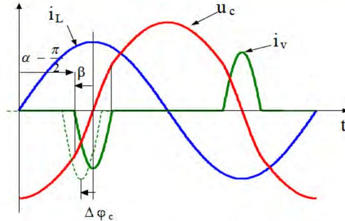
Figure 4-4. Capacitive Boost Mode
