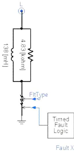
Figure 7-2. Fault Impedance
