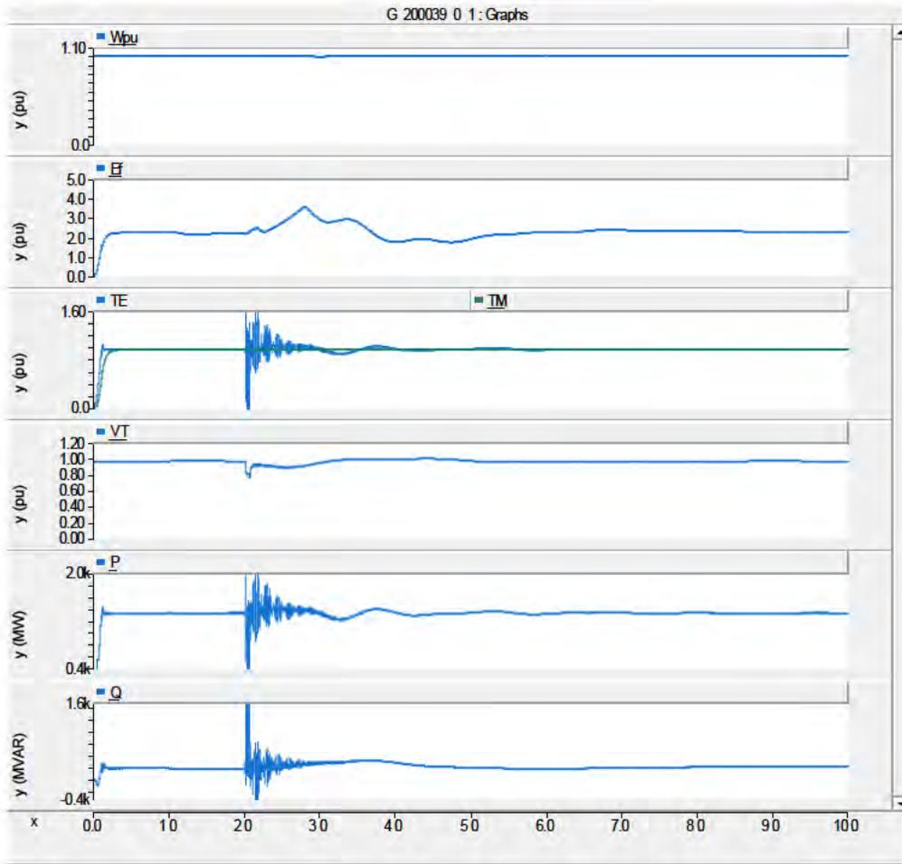
Figure 6-10. Transient Responses of Hope Creek Unit for Single Line to Ground Fault Simulation
