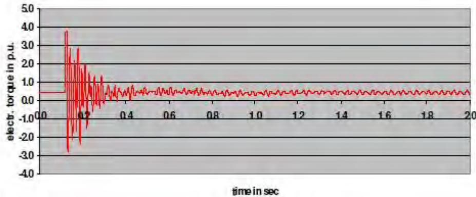
**Figure 3-3. Generator Air Gap Torque following a 3 Phase Fault**
