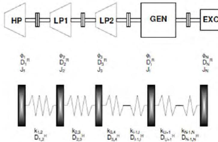
**Figure 3-1. Multi-Mass Rotor Model**
