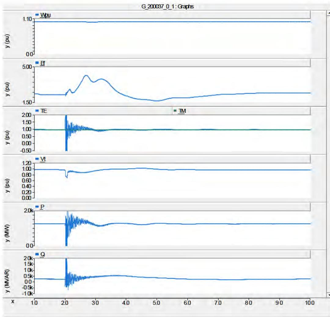
Figure 6-9. Transient Responses of Salem Unit 2 for Single Line to Ground Fault Simulation
