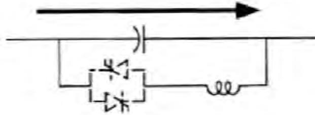
Figure 4-2. TCSC in Blocked Mode
