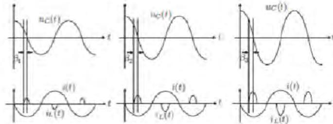
Figure 4-5. Variable TCSC Capacitive Reactance
