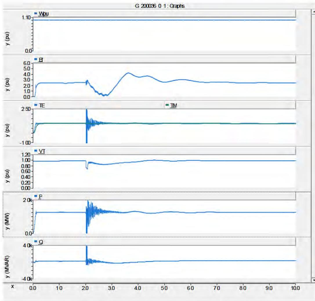
**Figure 6-8. Transient Responses of Salem Unit 1 for Single Line to Ground Fault Simulation**
