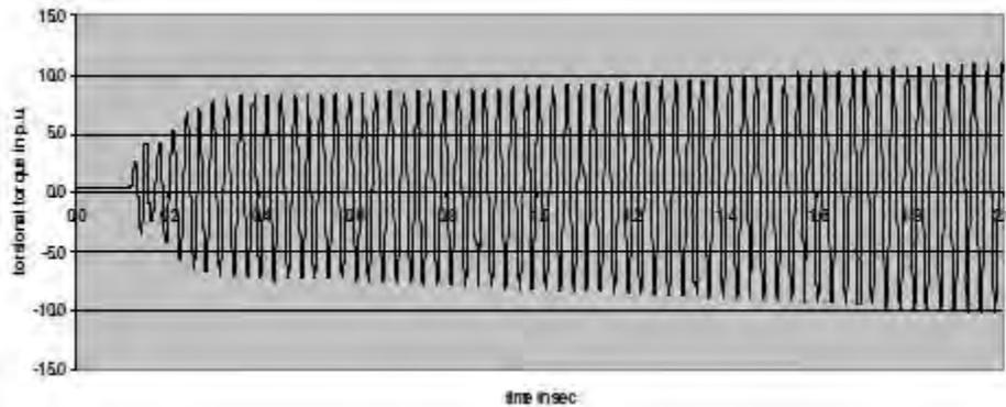
**Figure 3-4. Torque between Shaft Sections following a 3 Phase Fault**
