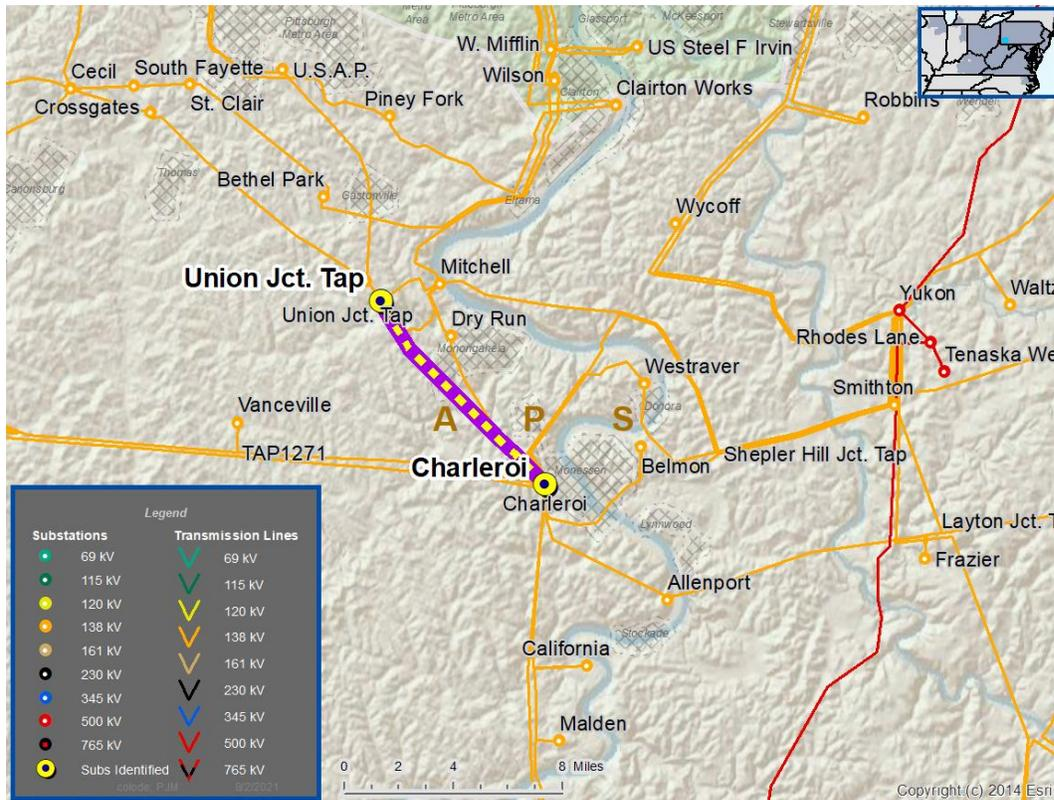
The recommended solution is to reconductor the Charleroi-Union Jct. 138 kV line and upgrade the terminal equipment at Charleroi 138 kV. The estimated cost for this project is \$11 million, with a required in-service date of June 2022. The projected in-service date is June 2023, and operating measures have been identified to mitigate reliability impacts in the interim. The local transmission owner, APS, will be designated to complete this work.
