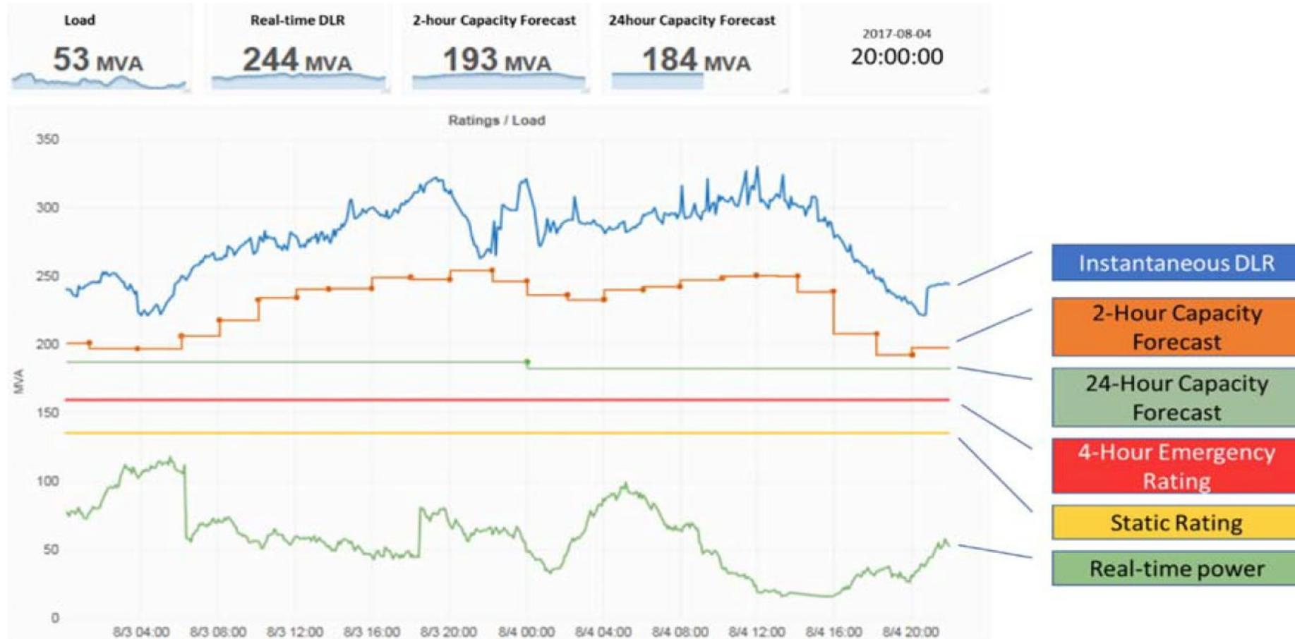
Figure 2: Transmission Capacity Forecast System Output showing 2- and 24-hour ahead forecasts
