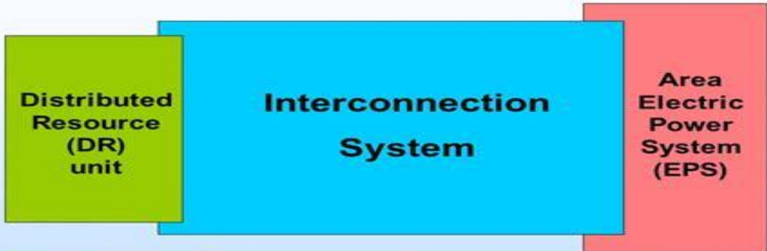
**IEEE Std 1547: Interconnection system requirements & specifications, and test requirements & specifications** 39
