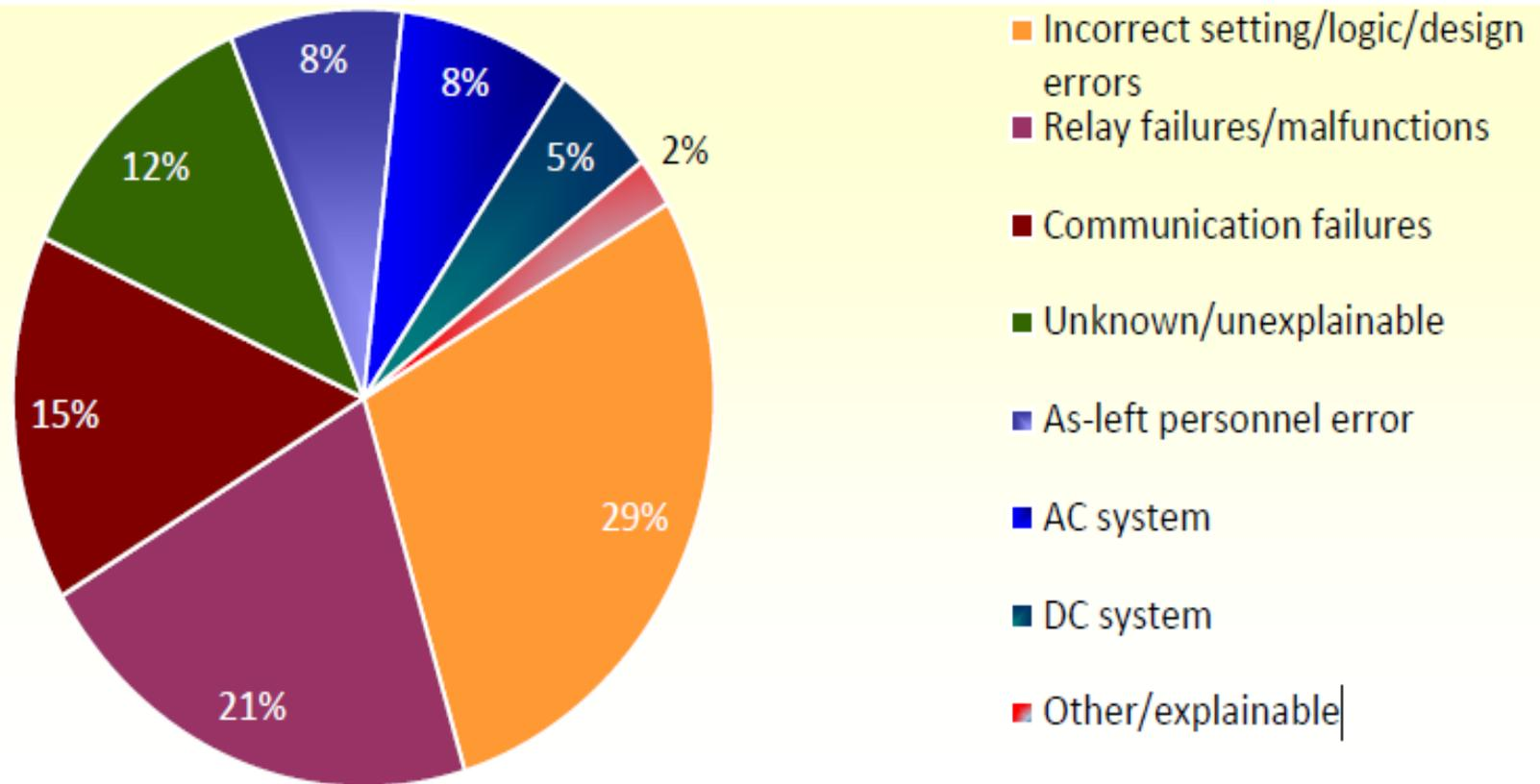
Figure 4.11: NERC Misoperations by Cause Code from 2011Q2 to 2013Q3<sup>70</sup>
