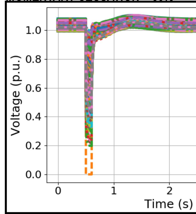
Complex Load, Central NJ fault, Voltage Regulation off, high feeder impedance, **transmission busses**
