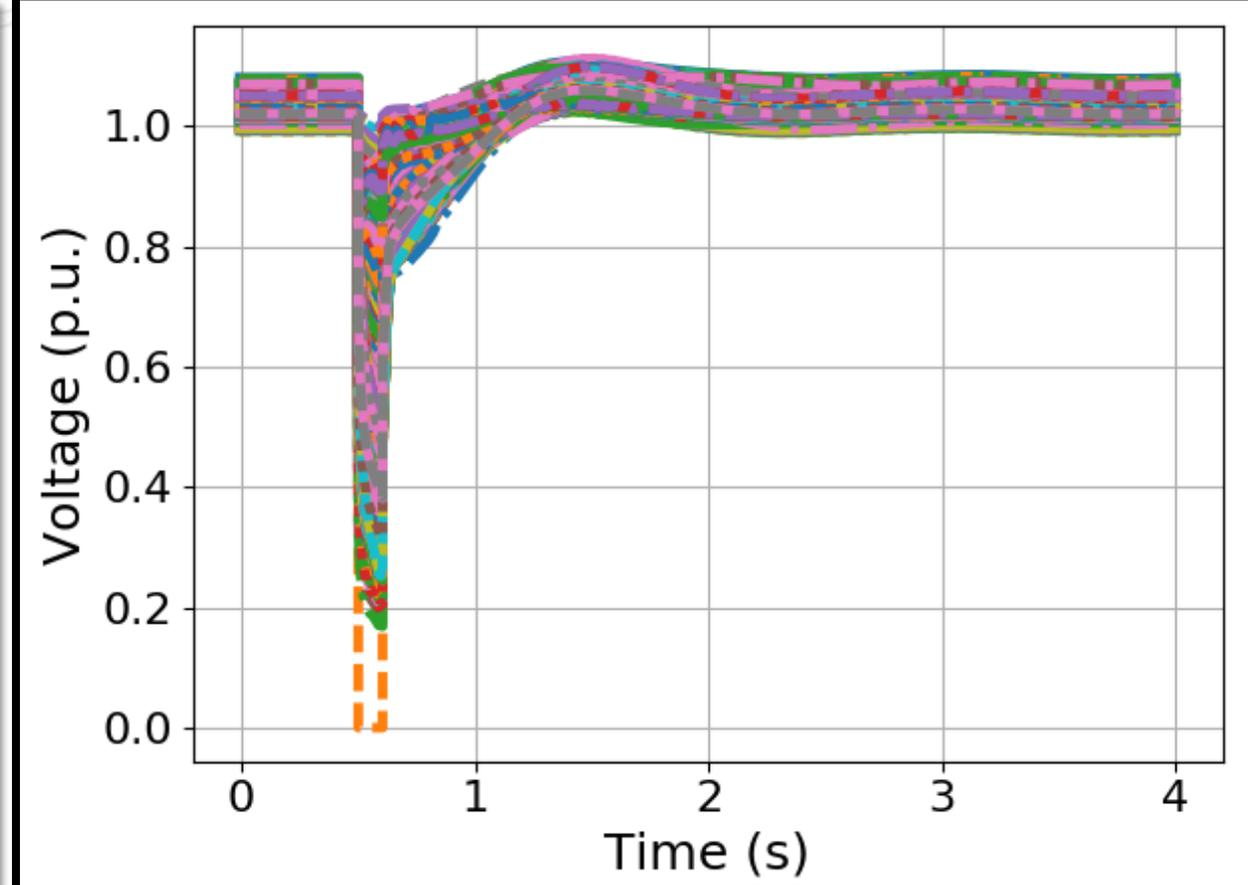
Complex Load, Central NJ fault, Voltage Regulation off, high feeder impedance, **transmission bus voltages**
