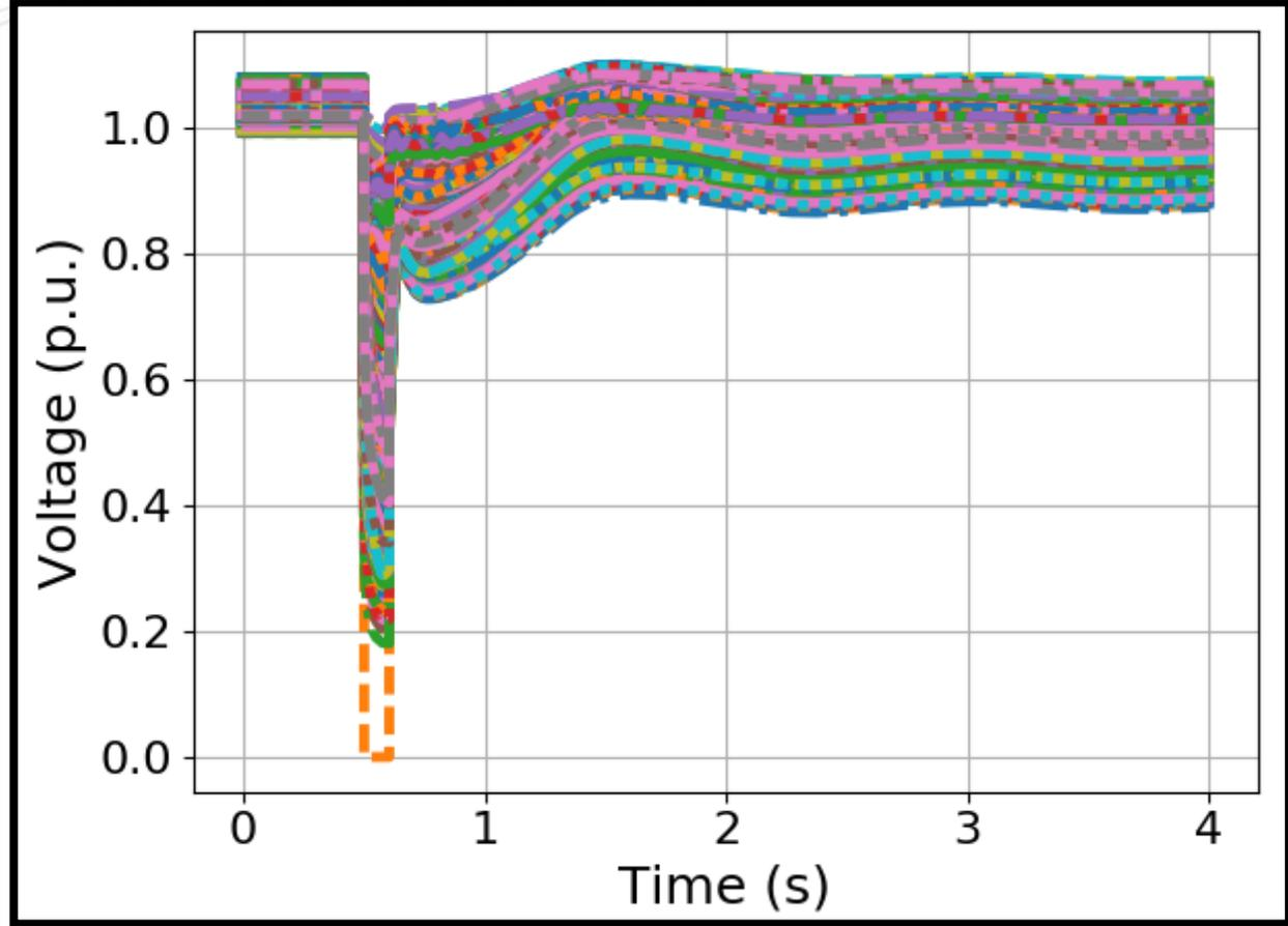
Complex Load, Central NJ fault, Voltage Regulation off, high feeder impedance
