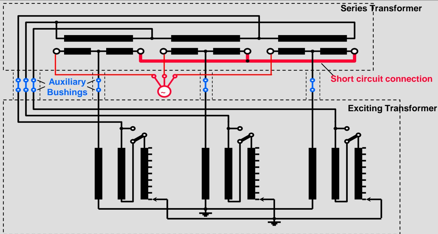
Temporary bushings inserted at all connections between series and exciting unit
