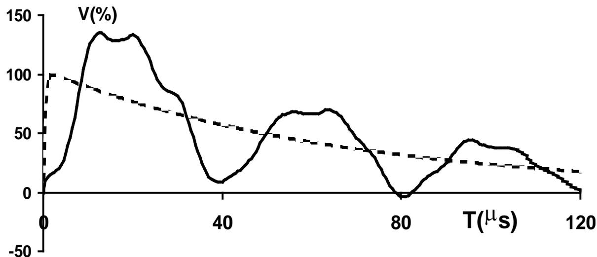
**Applied voltage and typical wave shape of voltage at crossover during lightning impulse test with source and load side terminals connected**
