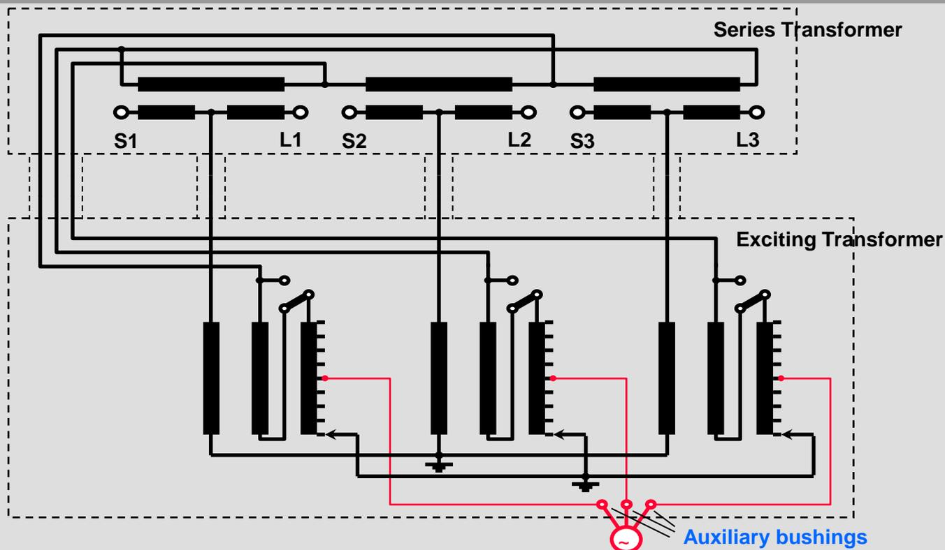
Temporary bushings are connected to the regulating winding
