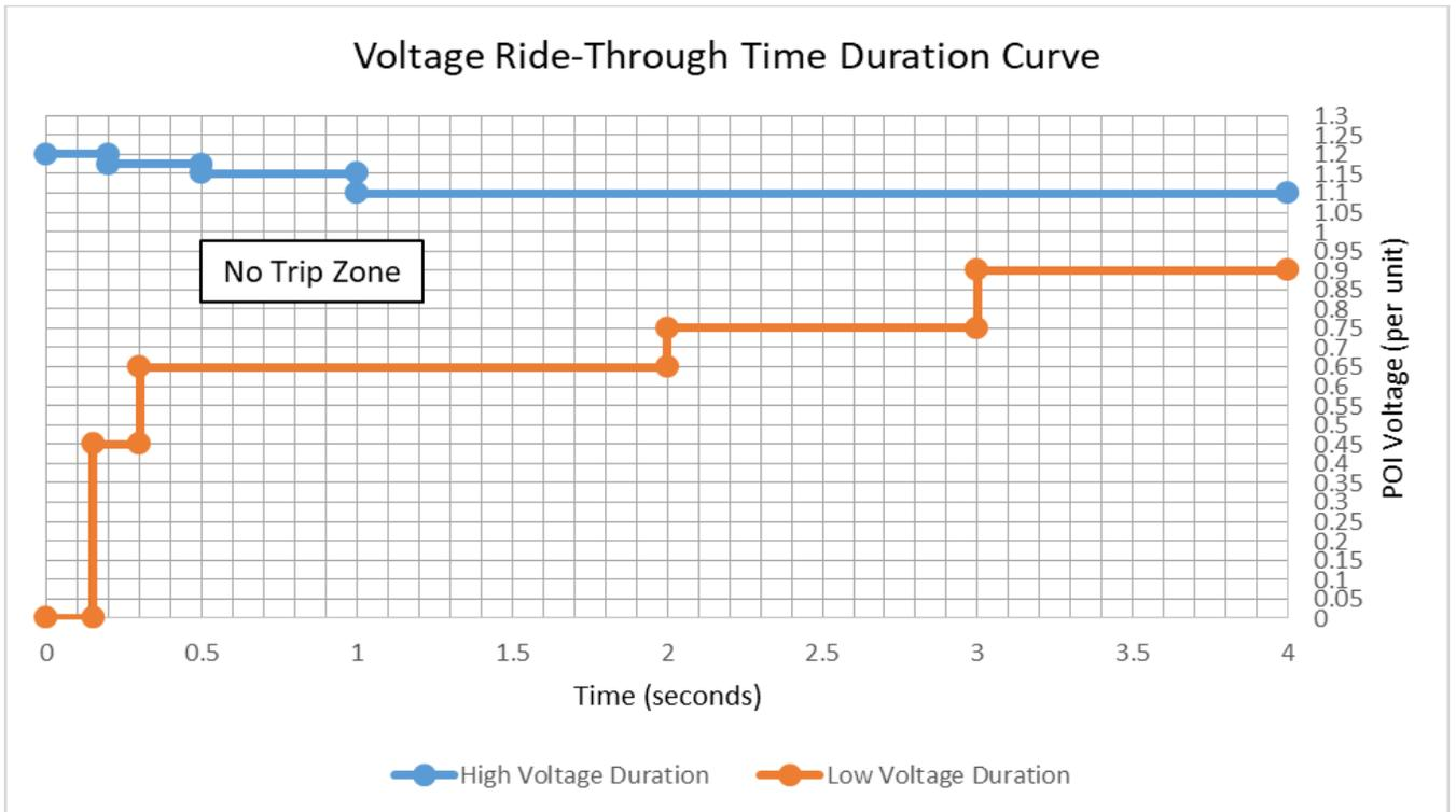
**Figure 7:** NERC Standard PRC-024 Voltage Ride-Through Duration Curve
