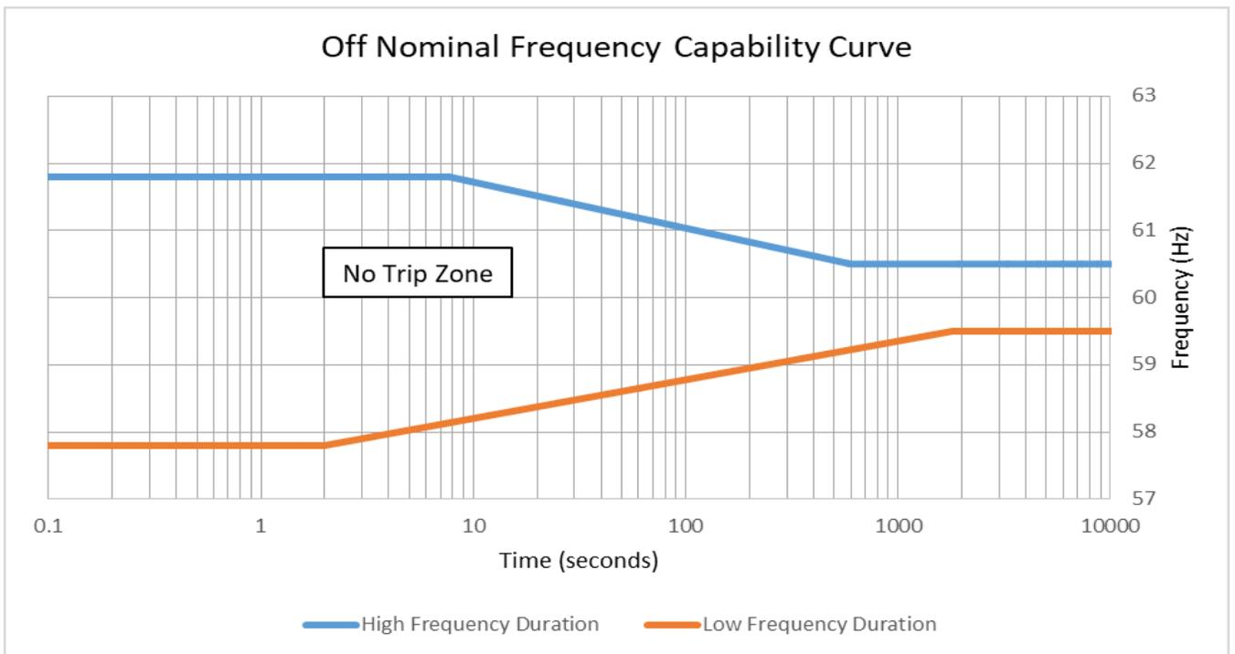
**Figure 8:** NERC Standard PRC-024 Frequency Ride-Through Capability Curve
