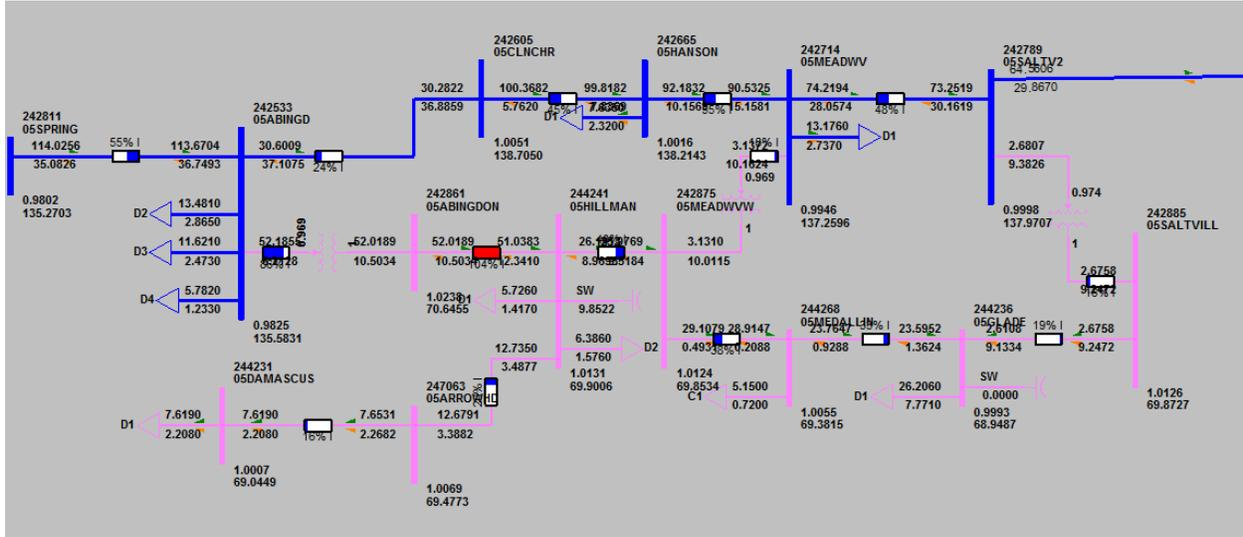
Figure D1: Loading on Abingdon – Hillman Hwy 69 kV Ckt 1 for the loss of Broadford – Sullivan 500 kV Ckt 1
