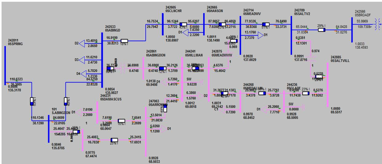
Figure D2: Loading on Abingdon – Hillman Highway 69 kV Ckt 1 for the loss of Broadford – Sulivan 500 kV Ckt 1 under this project
