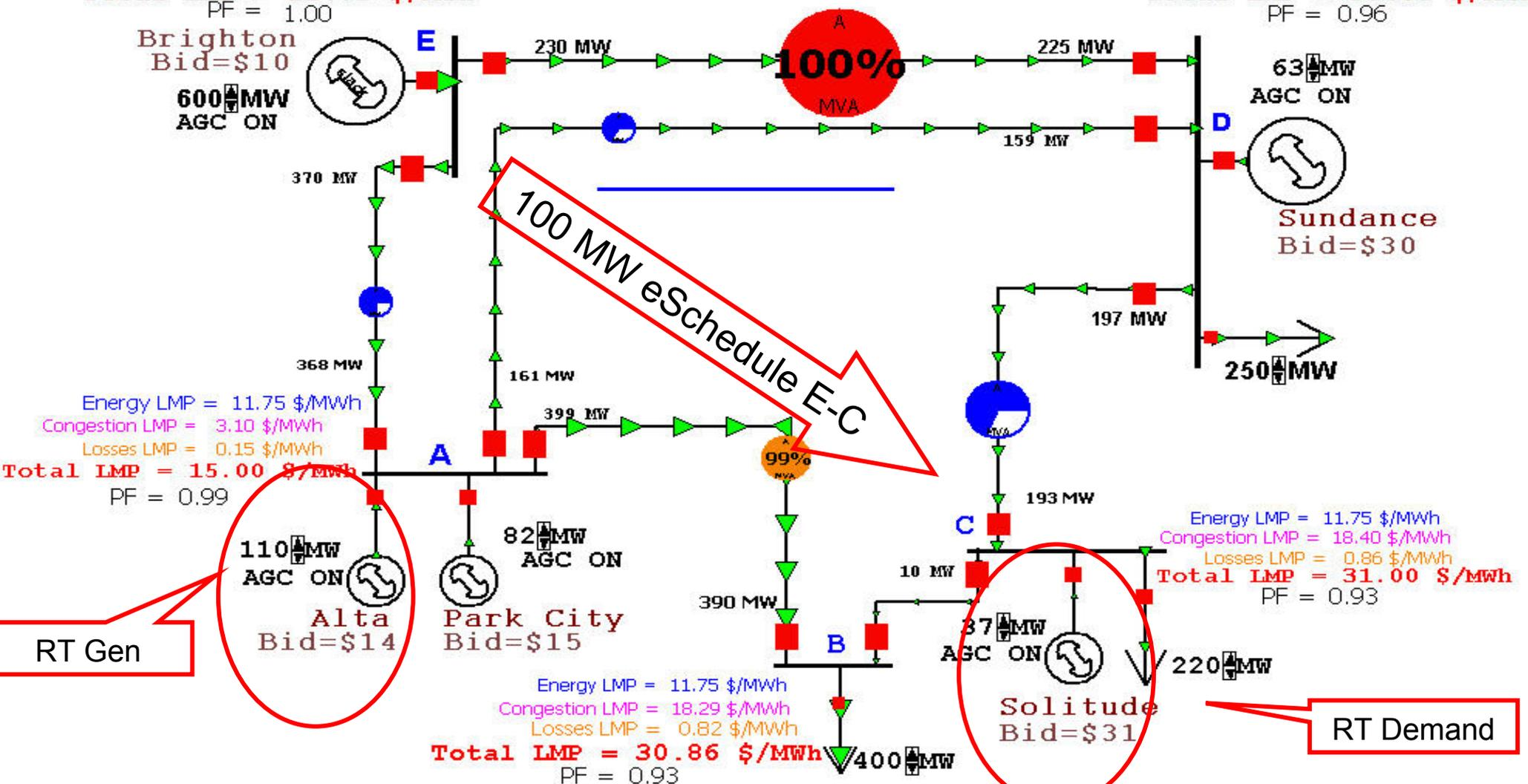
$$\text{Balancing Spot Market Charges} = \left[ \text{Real-Time Net Interchange (MWh)} - \text{Day-Ahead Net Interchange (MWh)} \right] * \text{Real-Time System Energy Price (\$/MWh)}$$
