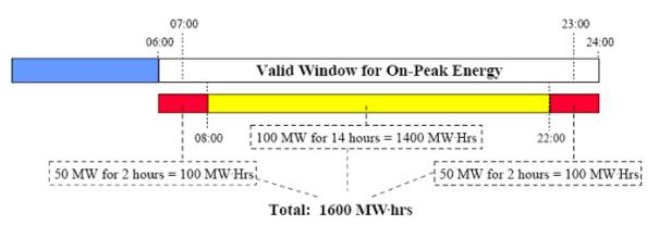
Example of Valid Energy Schedule using a 100MW Capacity
