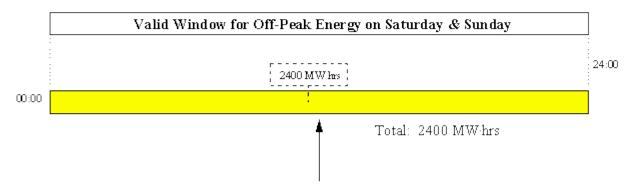
Example of Valid Energy Schedule using a 100MW Capacity Off-Peak Transmission Service Reservation
