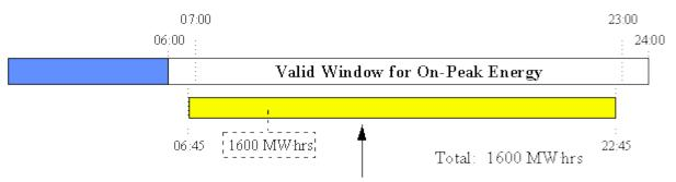
Example of Valid Energy Schedule using a 100MW Capacity
