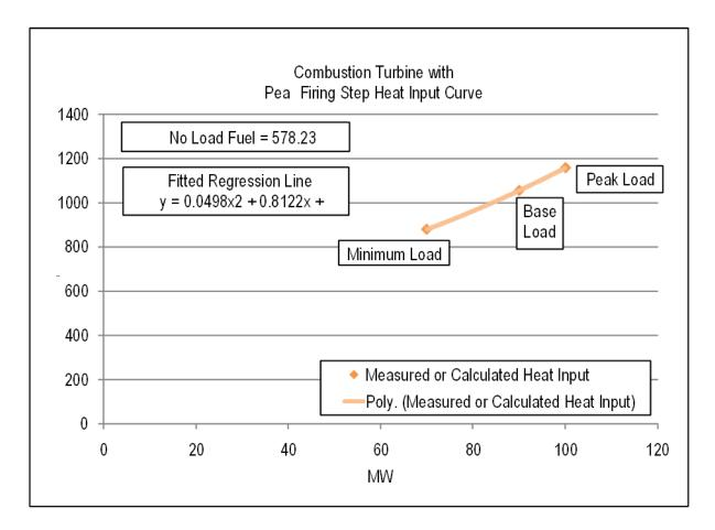
Each diamond in the graph above is a design heat input data point obtained from the original equipment manufacturer or calculated by heat balance. A regression analysis was performed on the design data to obtain the unit's Heat Input curve as a function of unit's output with natural gas as a fuel:
