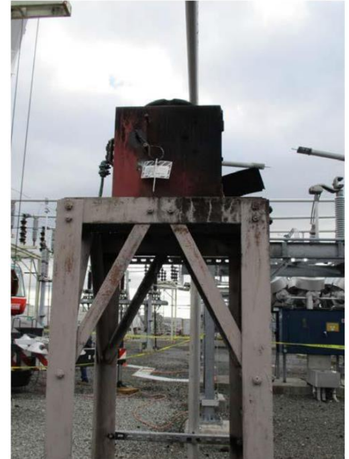
Figure 5: Failed C Phase CCPD [2]
