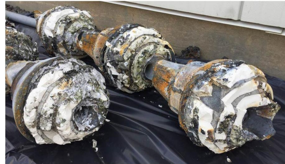
Figure 6: Remnants of Bus Insulators [2]
