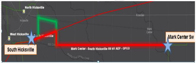
Existing Mark Center – South Hicksville 69 kV Line is highlighted in green; Proposed rebuild is highlighted in red.
