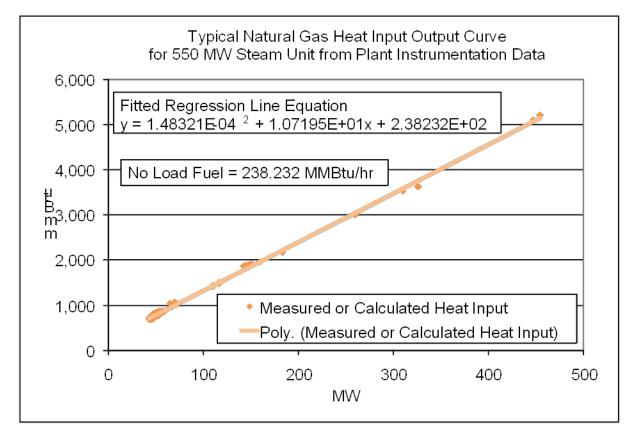
Each diamond in the graph above indicates one hourly heat input data point calculated from plant instrumentation during operations. A regression analysis was performed on the data collected to obtain the unit's Heat Input curve as a function of various unit output levels with oil as a fuel:
