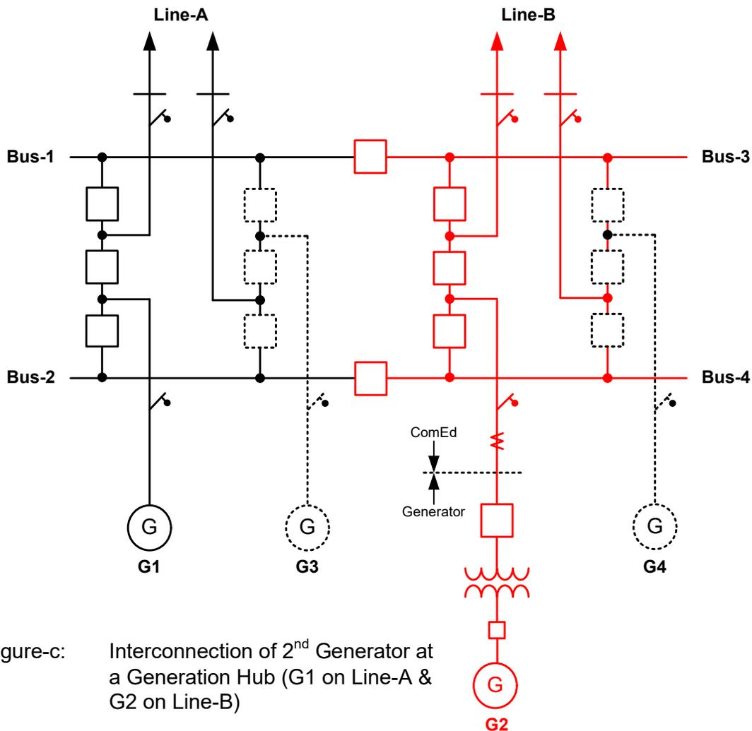
Figure-c: Interconnection of 2<sup>nd</sup> Generator at a Generation Hub (G1 on Line-A & G2 on Line-B)
