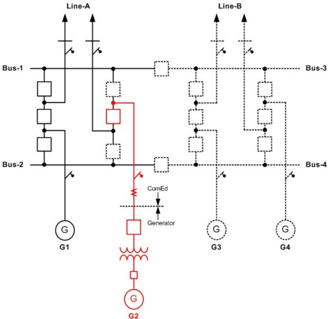
Figure-b: Interconnection of 2<sup>nd</sup> Generator at a Generation Hub (G1 on Line-A & G2 on Line-A)
