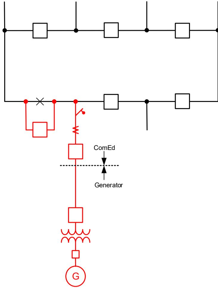
Figure-3.1.1: Generator interconnection to an existing nuclear station
