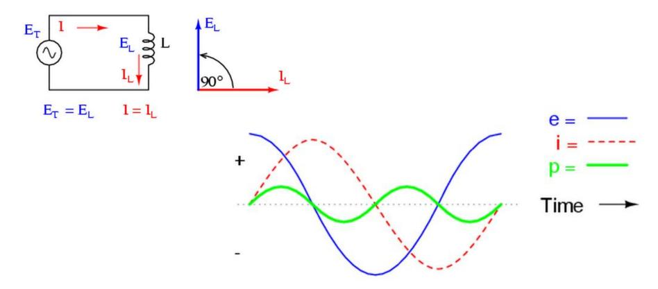
Calculate the inductive reactance of a circuit having a pure inductance of 50 millihenries with a frequency of 60 Hz.
