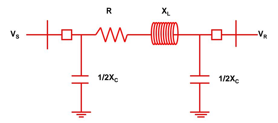
Values will depend on a line's length, cross-sectional area, and conductor spacing
