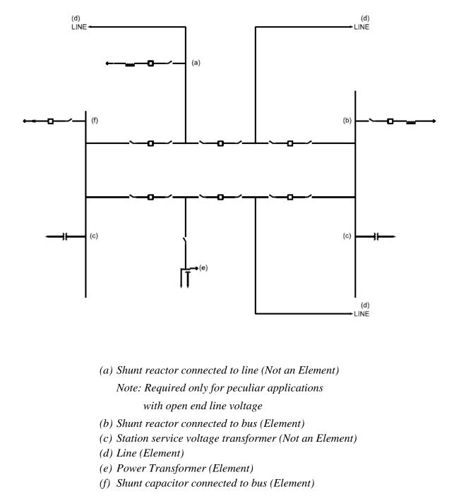
Figure 1 - One-Line diagram showing elements and non-elements
