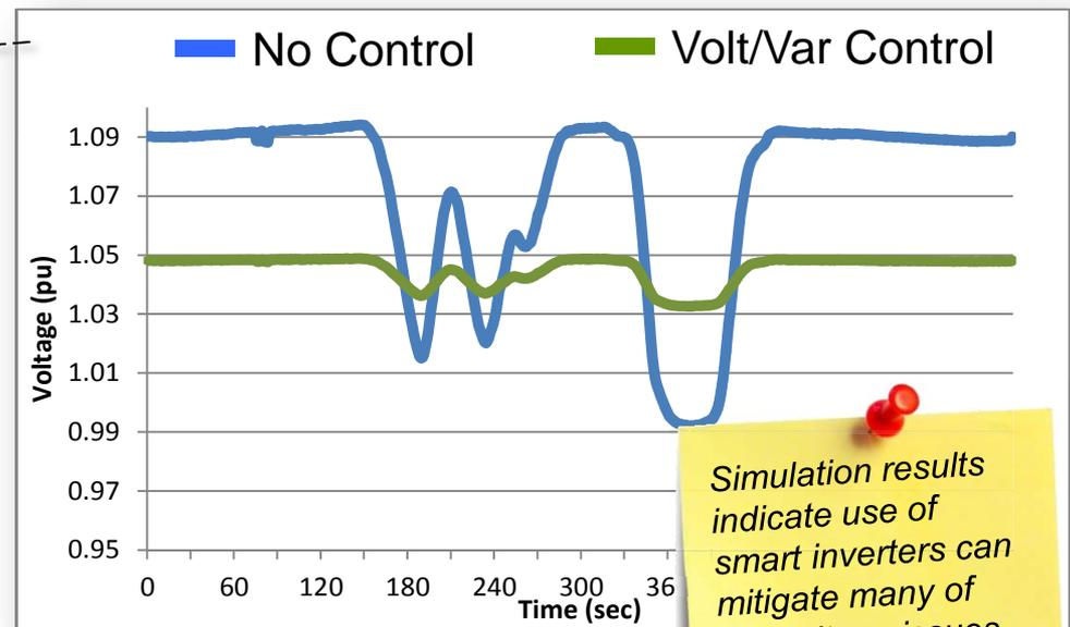
Simulation results indicate use of smart inverters can mitigate many of the voltage issues resulting from PV
