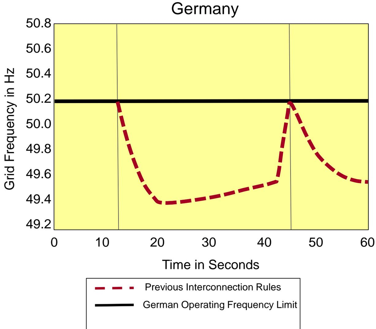
As of 2012 PV Inverters were not required to provide frequency support and disconnect from the grid if the frequency reaches 50.2 Hz
