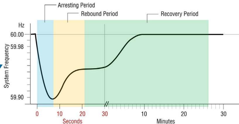
VG may displace conventional units & **reduce system inertia & primary frequency response**
