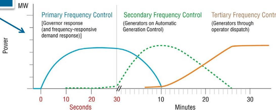
Non-synchronous VG may **provide inertia & primary frequency response through power electronics**
