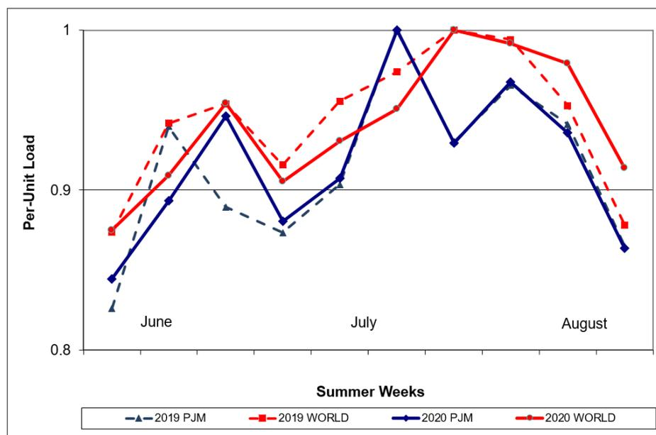
Figure II-4 shows the weekly share of Loss of Load for the PJMRT0 in the 2019 RRS and 2020 RRS. No major differences in the weekly share of LOLE are observed between the two studies except for a slight shift of LOLE risk from July to August.
