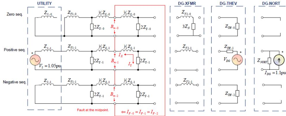
Figure 2. Sequence networks for a SLGF at feeder midpoint, with wye impedance grounded/delta interconnection transformer shown and either a Thevenin or Norton DG equivalent.
