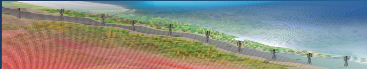
**Computational Fluid Dynamics (CFD)** used to model Numerical Weather Prediction wind speeds at **each individual span**, based on local topography and vegetation.
