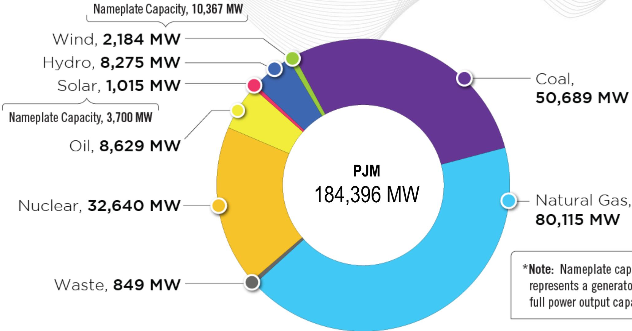
**\*Note:** Nameplate capacity represents a generator's rated full power output capability.
