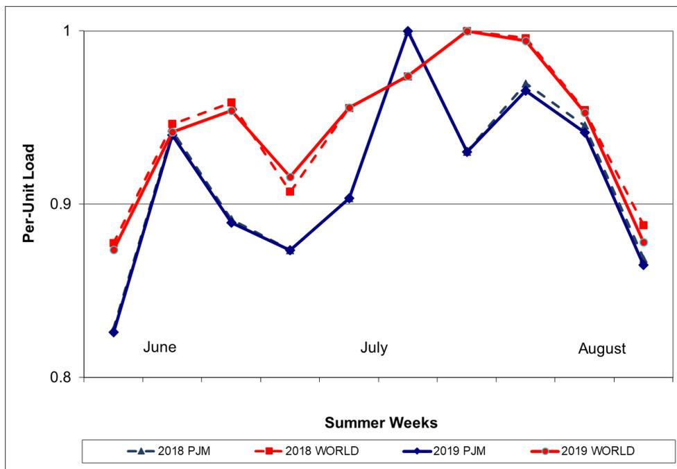
Figure II-4 shows the weekly share of Loss of Load for the PJM RTO in the 2018 RRS and 2019 RRS. No major differences in the weekly share of LOLE are observed between the two studies.
