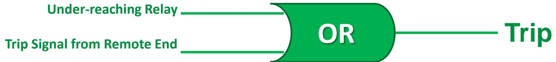
**OR:** Needs one high input in order to provide an output
