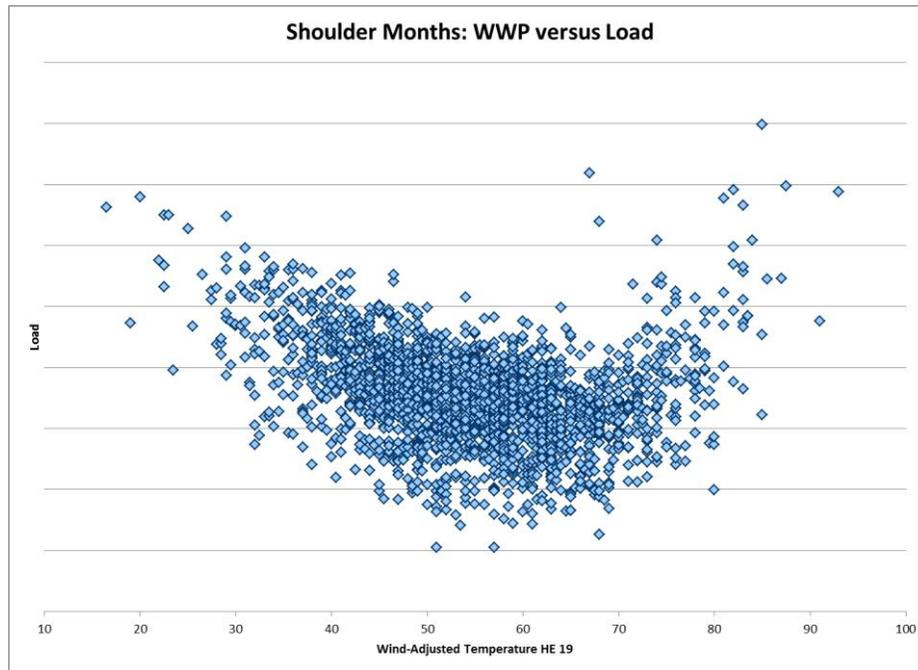
To accommodate this situation, the load to weather relationship is permitted to vary over three segments (see Figure IV-7). In doing so, the model can account for conditions that mimic winter or summer, as well as mild conditions in which there is little weather sensitivity.
