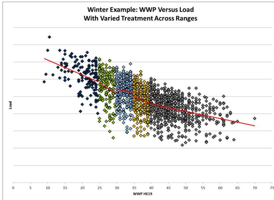
Weather conditions vary across the PJM footprint so it is best to treat zones individually, recognizing that what characterizes extreme conditions can vary zone by zone. Spline cut-off points were selected with the goal of best representing the behavior of load under extreme weather conditions when seasonal peaks will occur. The process to accomplish this was as follows:
