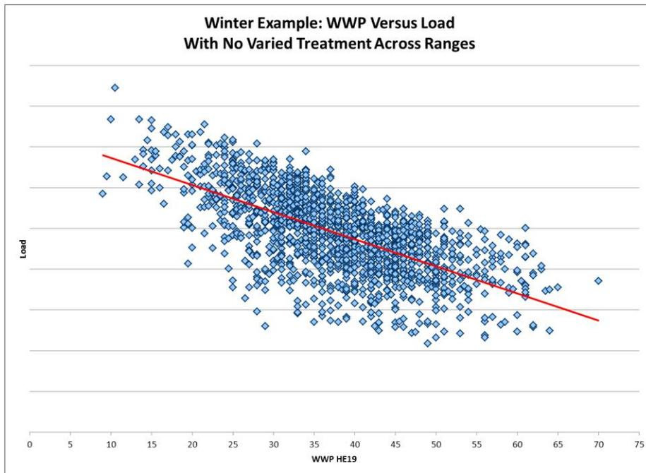
A better representation of the load to weather relationship is to allow for a different load response at different ranges of the given weather variable. There are mild days that elicit minimal load-weather response. Also, there is some degree of HVAC saturation in extreme weather (i.e. the load to weather response moderates as equipment operates constantly).
