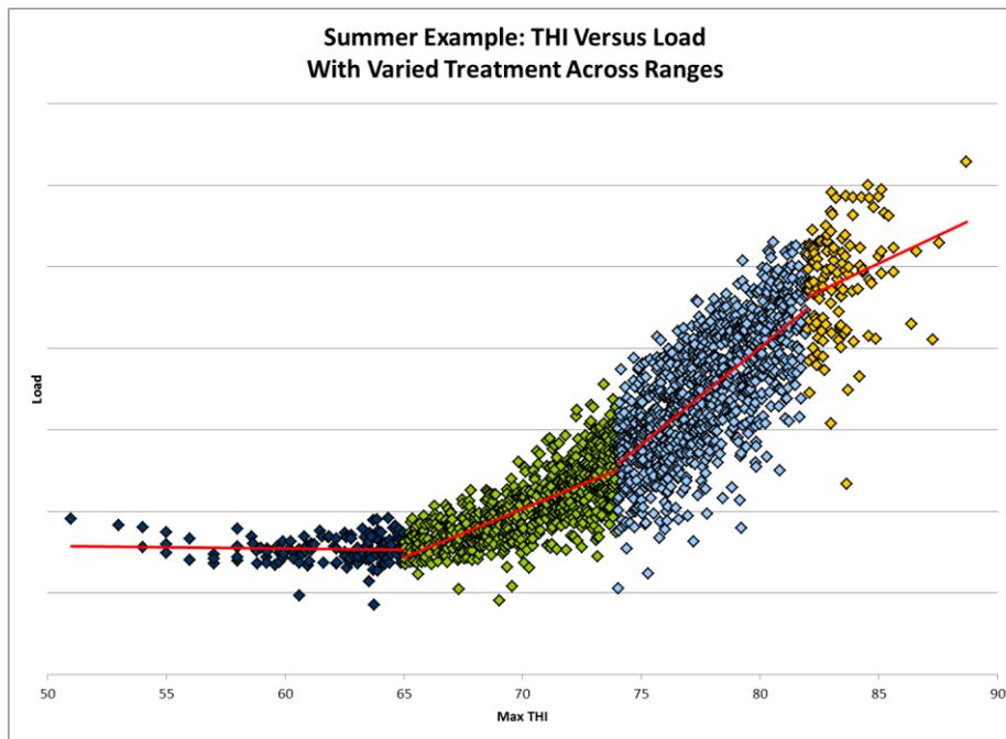
Figure IV-5 : WWP Example (Granular Treatment)
