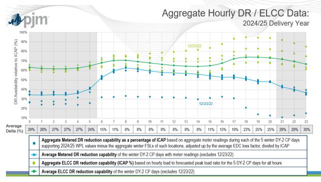
Presented at the Aug. 7 MIC, the figure above compares the estimated reduction capability of DR based on the aggregate hourly metered loads of customers during the 5 winter peak days minus winter FSL (in blue) to the reduction capability used in the ELCC analysis during those same days (in green), as a percentage of winter ICAP for the 2024/25 DY. ELCC heuristic (in green) shown for all hours, but zero reduction value used in analysis during the shaded hours outside current performance window.
