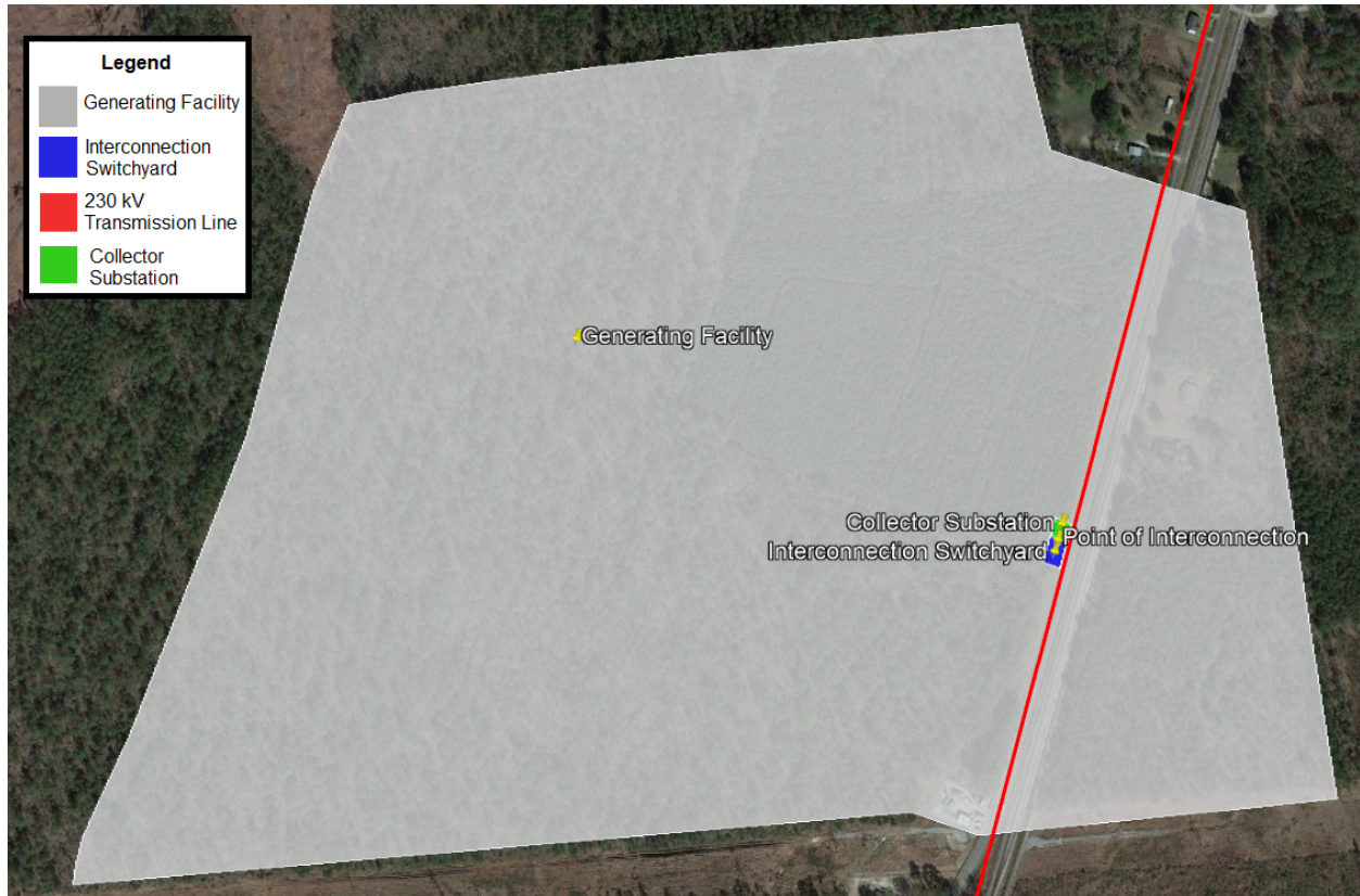
Exhibit 46: Tapping an Existing Transmission Line
