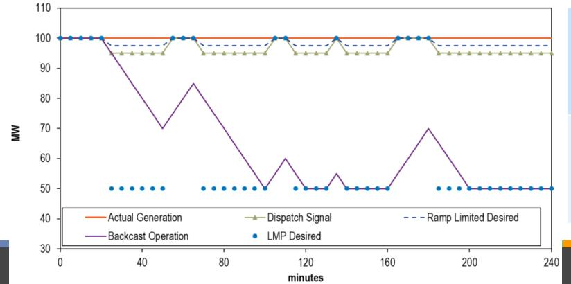
Compared to the dispatch signal or Ramp Limited Desired, actual generation is close to the desired MW and the unit looks like it is following dispatch
