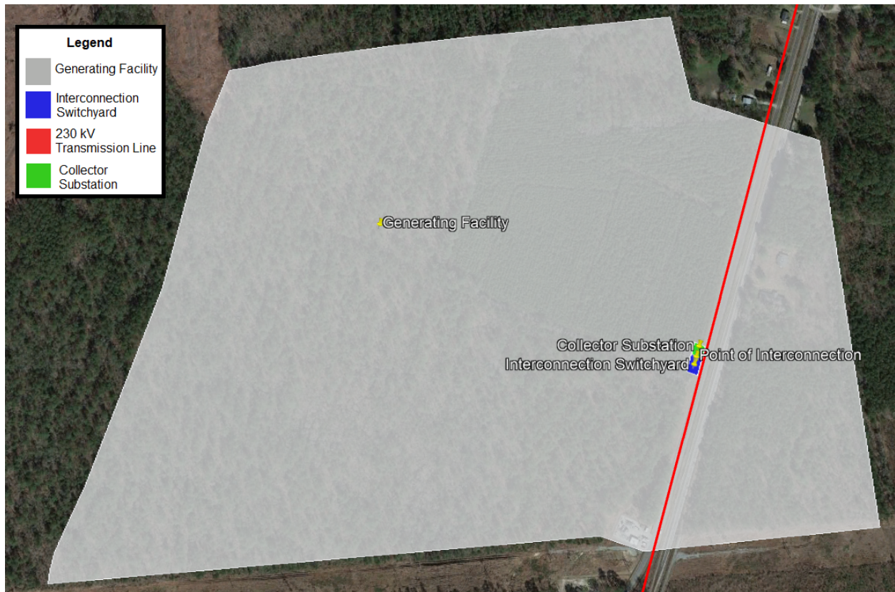
Exhibit 50: Tapping an Existing Transmission Line
