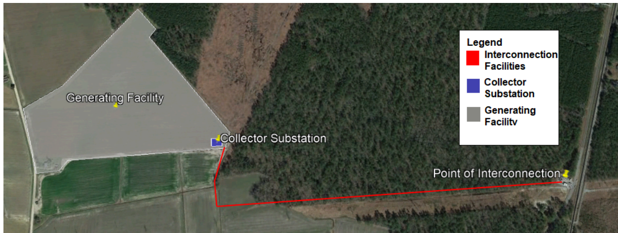
Exhibit 50: Interconnecting into an Existing Substation
