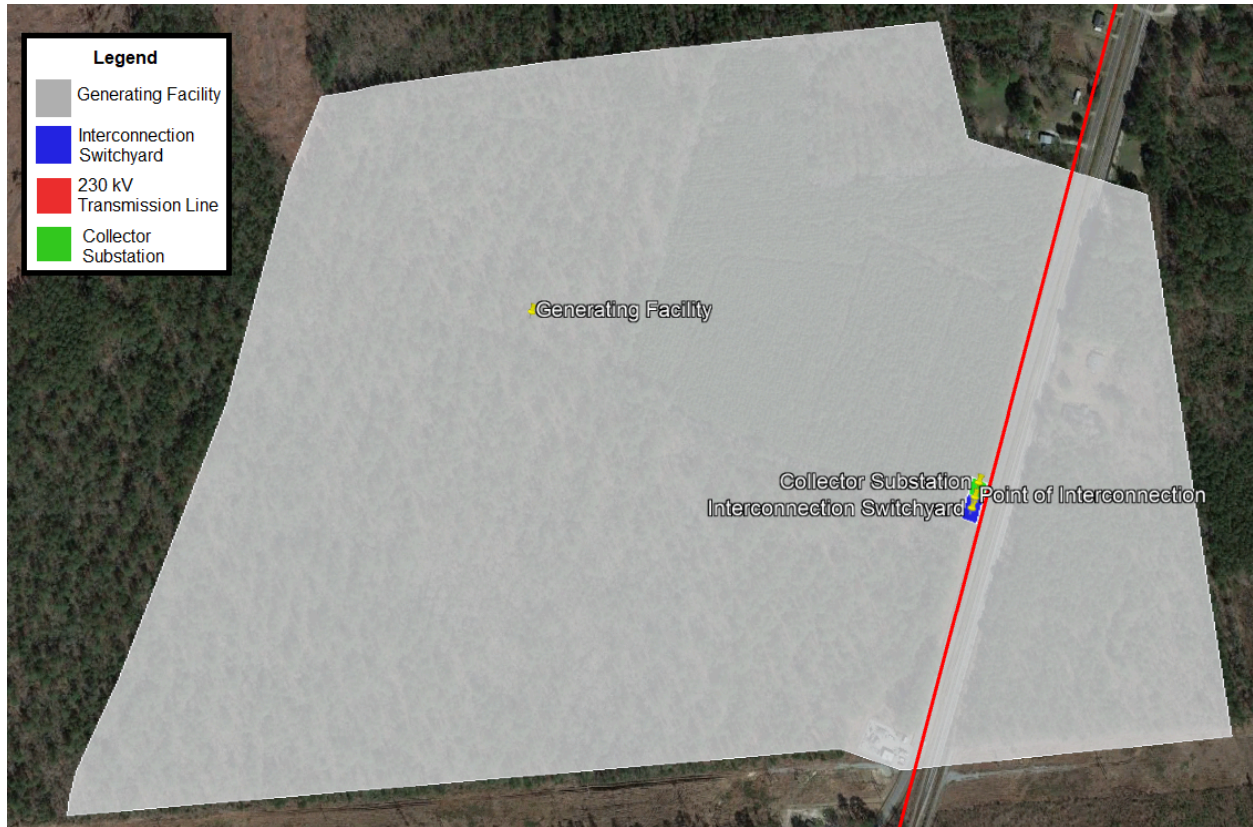
Exhibit 50: Tapping an Existing Transmission Line
