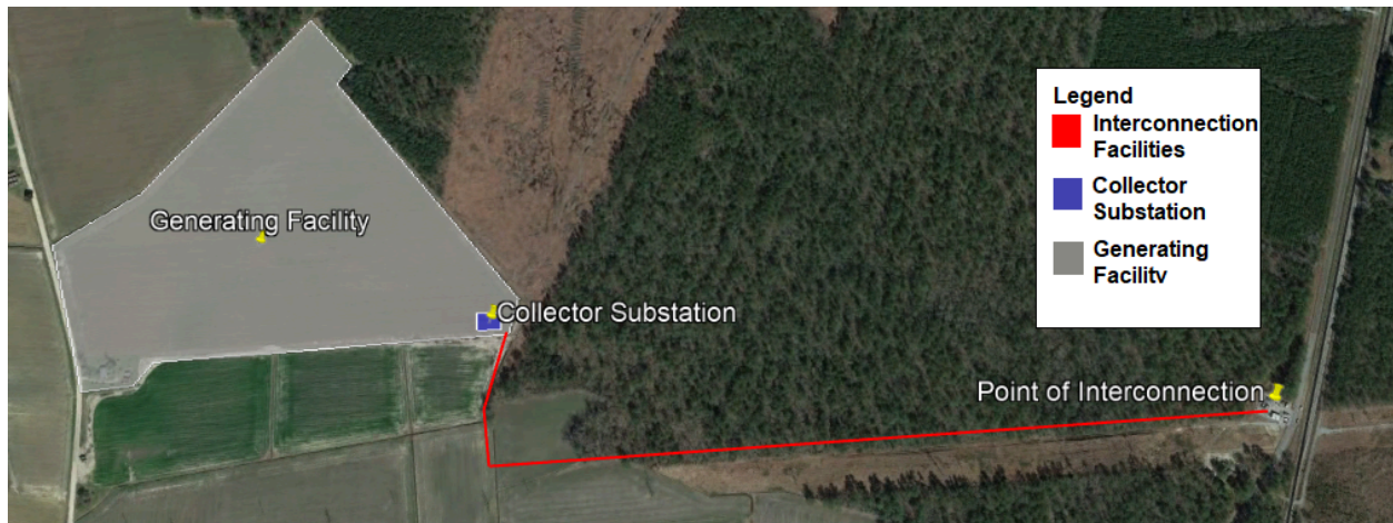
Exhibit 46: Interconnecting into an Existing Substation
