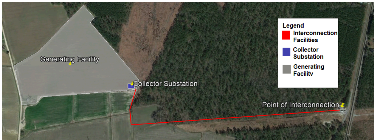
Exhibit 48: Interconnecting into an Existing Substation
