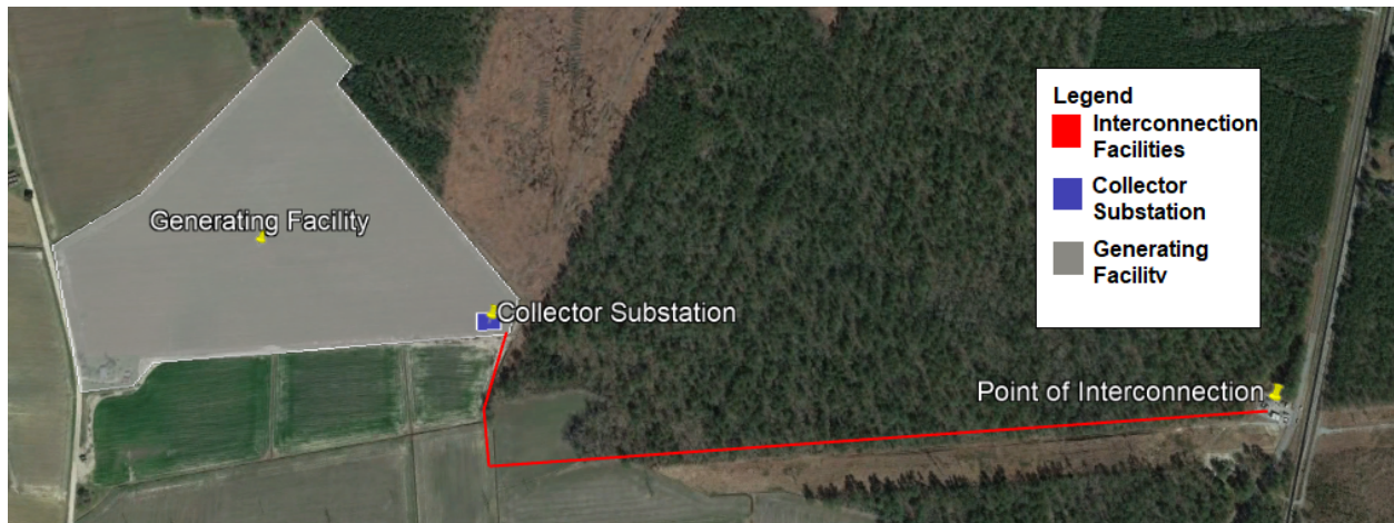
Exhibit 49: Interconnecting into an Existing Substation
