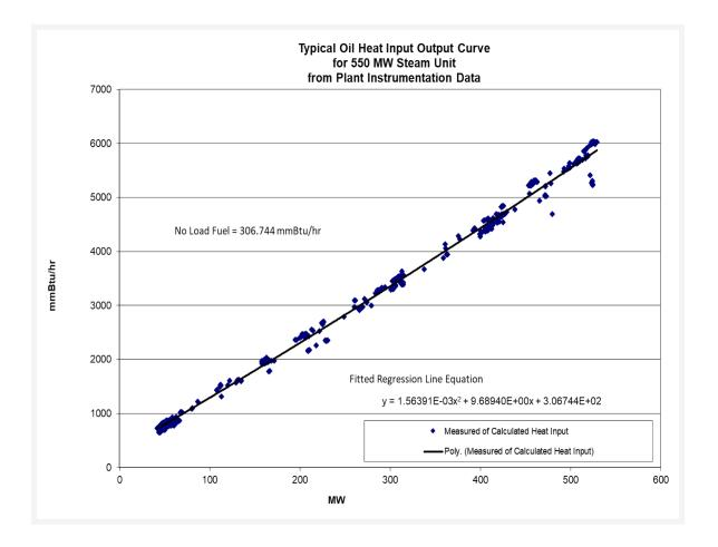
Each diamond in the graph above indicates one hourly heat input data point calculated from plant instrumentation during operations. A regression analysis was performed on the data collected to obtain the unit's Heat Input curve as a function of unit's output with oil as a fuel:
