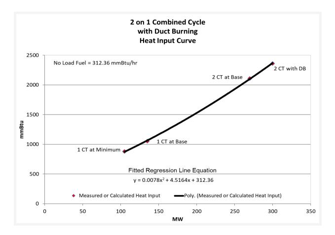
Each diamond in the graph above is a design heat input data point obtained from the original equipment manufacturer or calculated by heat balance. A regression analysis was performed on the design data to obtain the unit's Heat Input curve as a function of unit output levels with natural gas as a fuel:
