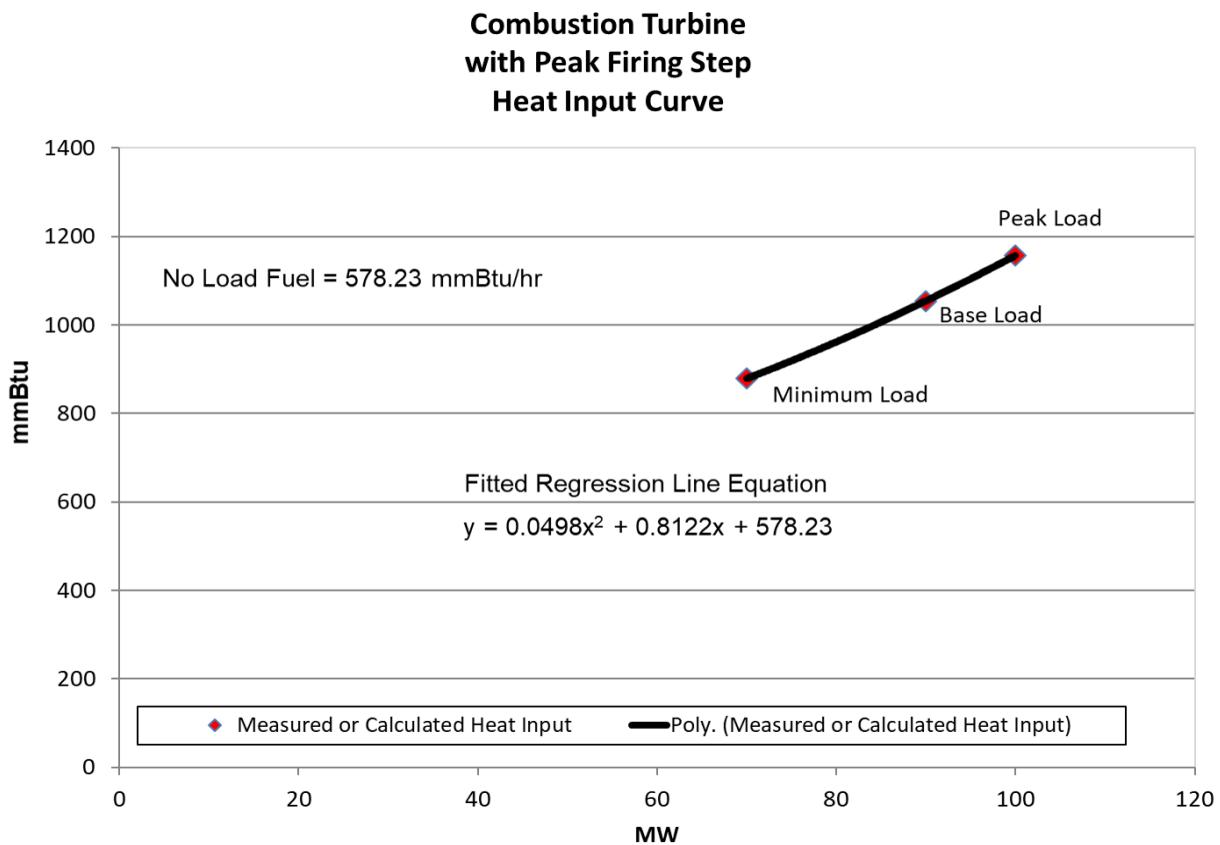
Each diamond in the graph above is a design heat input data point obtained from the original equipment manufacturer or calculated by heat balance. A regression analysis can be performed on the design data to obtain the unit's Heat Input curve as a function of various unit output levels with natural gas as a fuel:
