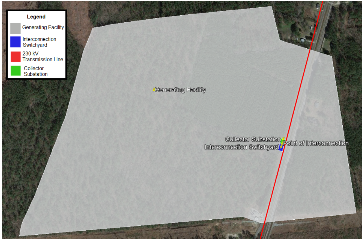
Exhibit 47: Tapping an Existing Transmission Line
