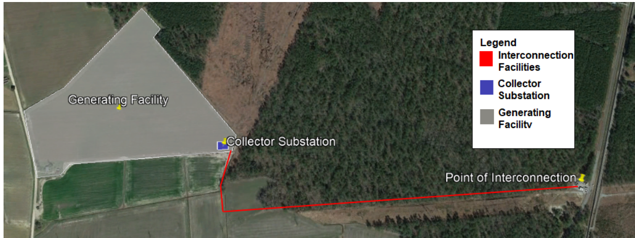
Exhibit 46: Interconnecting into an Existing Substation
