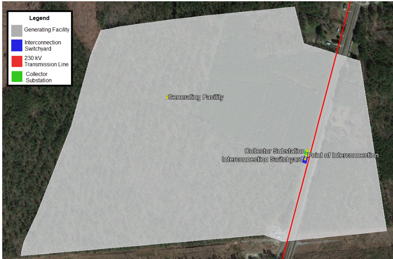
Exhibit 47: Tapping an Existing Transmission Line
