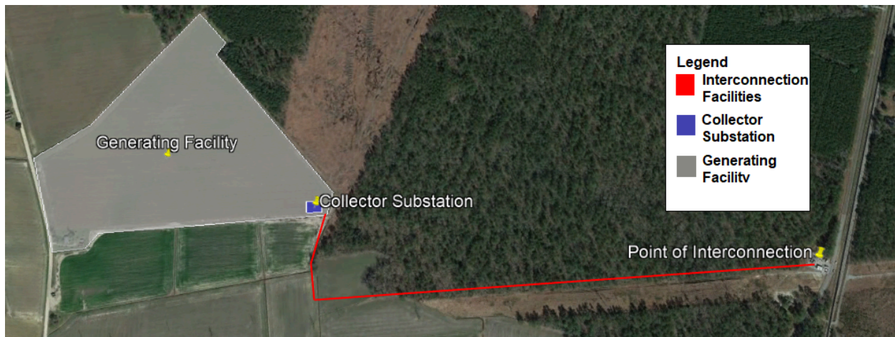
Exhibit 45: Interconnecting into an Existing Substation
