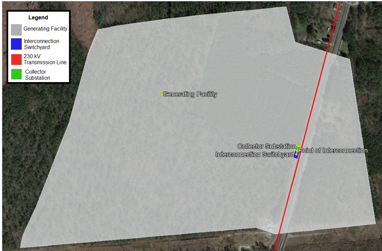
Exhibit 46: Tapping an Existing Transmission Line
