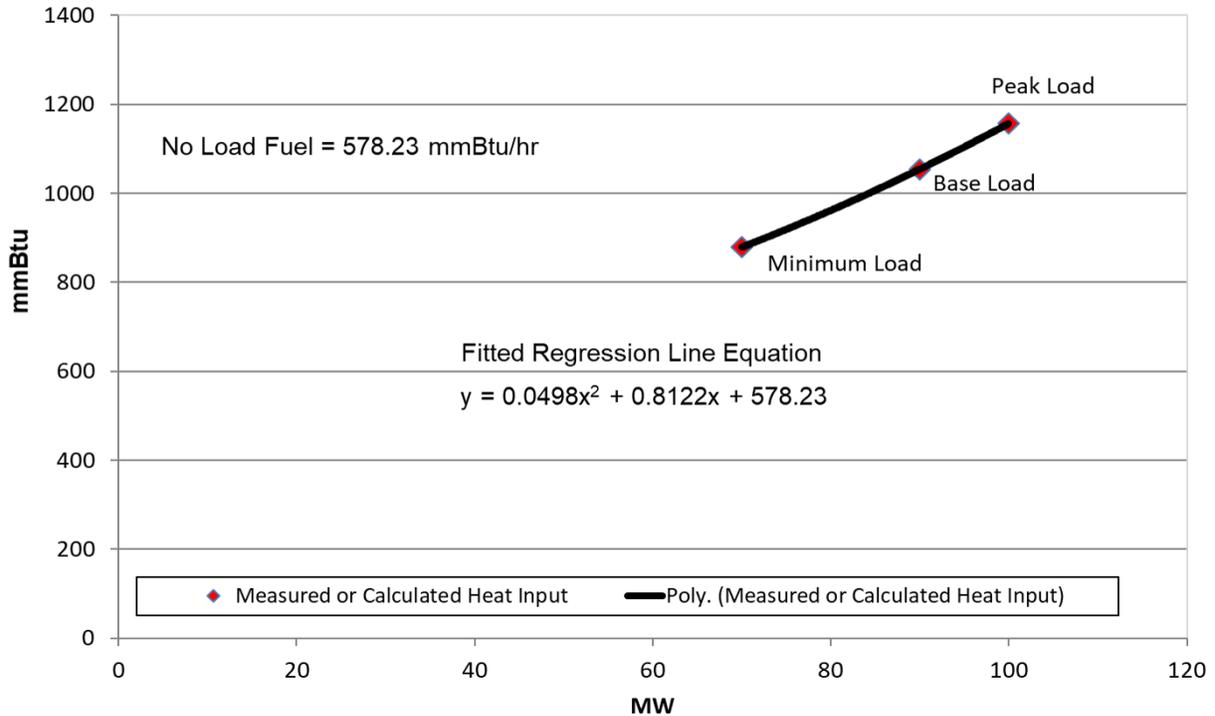
Each diamond in the graph above is a design heat input data point obtained from the original equipment manufacturer or calculated by heat balance. A regression analysis was performed on the design data to obtain the unit's Heat Input curve as a function of unit's output with natural gas as a fuel:
