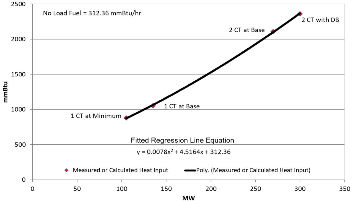
Each diamond in the graph above is a design heat input data point obtained from the original equipment manufacturer or calculated by heat balance. A regression analysis was performed on the design data to obtain the unit's Heat Input curve as a function of unit output levels with natural gas as a fuel:
