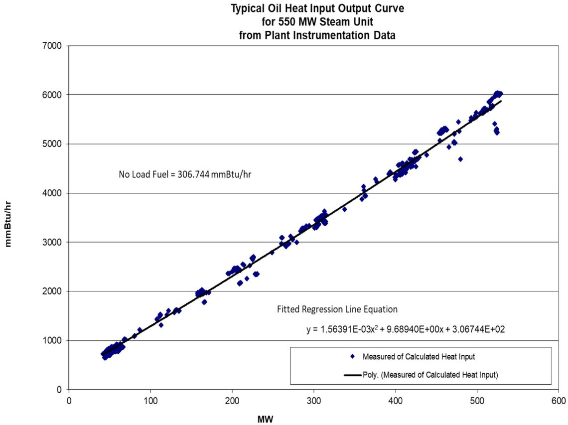
Each diamond in the graph above indicates one hourly heat input data point calculated from plant instrumentation during operations. A regression analysis was performed on the data collected to obtain the unit's Heat Input curve as a function of unit's output with oil as a fuel:
