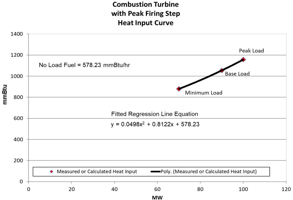
Each diamond in the graph above is a design heat input data point obtained from the original equipment manufacturer or calculated by heat balance. A regression analysis can be performed on the design data to obtain the unit's Heat Input curve as a function of various unit output levels with natural gas as a fuel:
