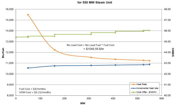
Typical Natural Gas Heat Rate & Cost Curves for 550 MW Steam Unit
