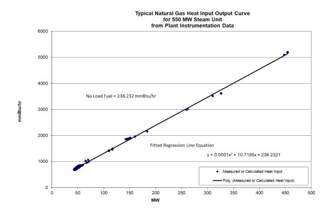
Each diamond in the graph above indicates one hourly heat input data point calculated from plant instrumentation during operations. A regression analysis was performed on the data collected to obtain the unit's Heat Input curve as a function of various unit output levels with oil as a fuel:
