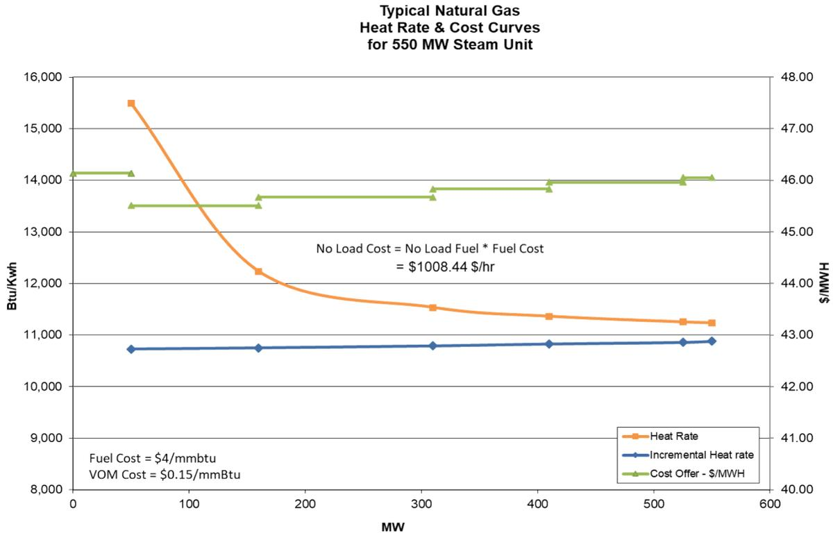
The ~~N~~o-~~L~~oad ~~c~~Cost was then raised to \$1007.76 until the first increment of the cost offer was less than \$1/MWh below the second increment, producing a monotonically increasing curve in the graph below:
