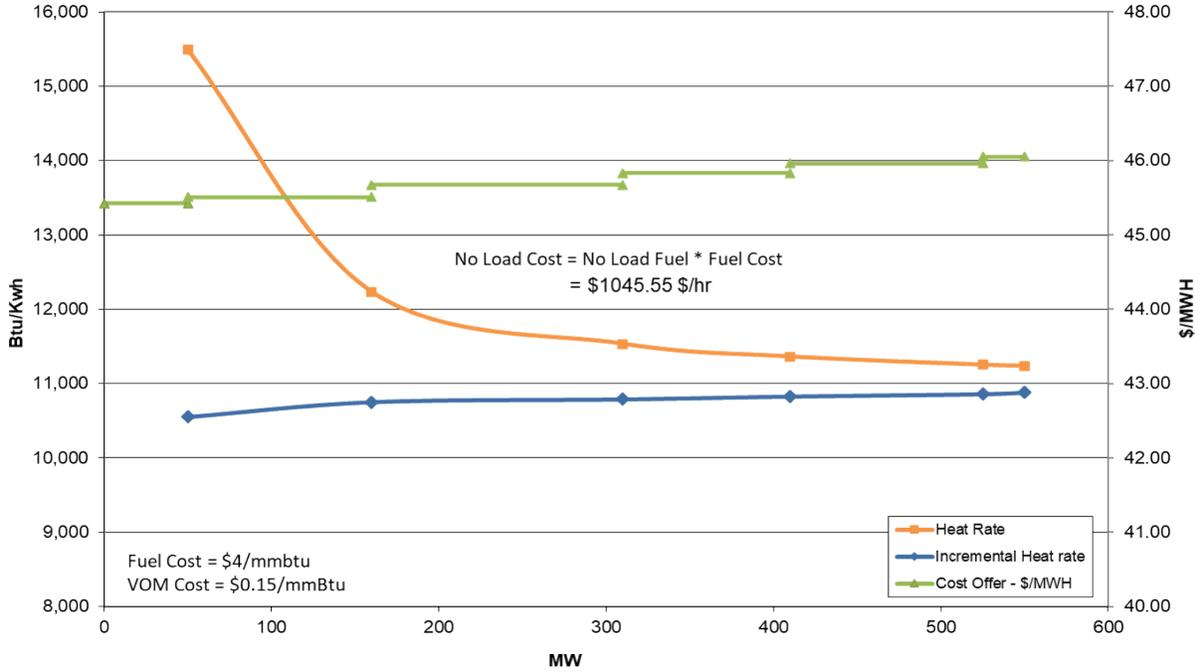
To avoid making adjustments to the ~~nNo-Load cG~~Cost, first calculate the unit's Incremental Cost (\$/MWh) at various outputs using the derivative of the Heat Input Curve:
