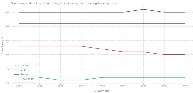
ELCC Class Ratings for Coal, Nuclear, Steam and Diesel Utility for period DY 2027 - DY 2035
