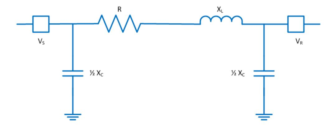
Values will depend on a line's length, cross-sectional area, and conductor spacing
