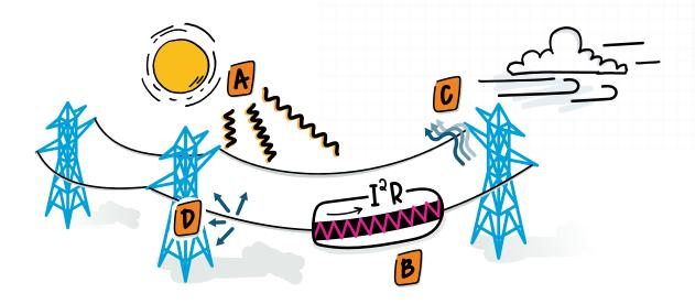
Dynamic Line Rating (DLR) technology uses advanced sensors and software to monitor real-time conductor temperature along a transmission line.
