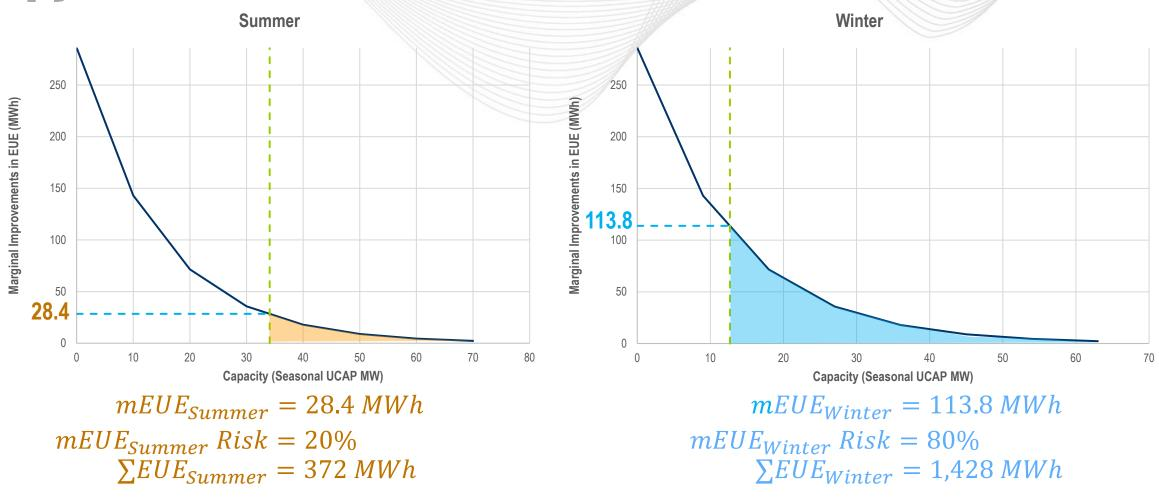
$EUE_{Annual} = 372 \ MWh + 1,428 \ MWh = 1,800 \ MWh$
