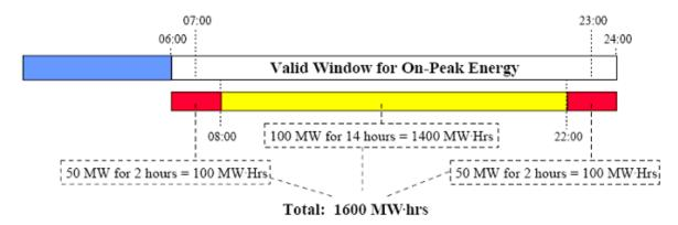
Example of Valid Energy Schedule using a 100MW Capacity On-Peak Transmission Service Reservation Over 18 Hour Period
