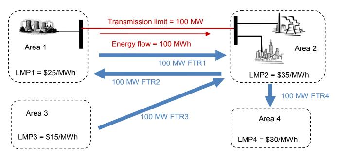
Figure 10 - Simple Electricity System with Congestion (National Energy Technology Laboratory 2013)
