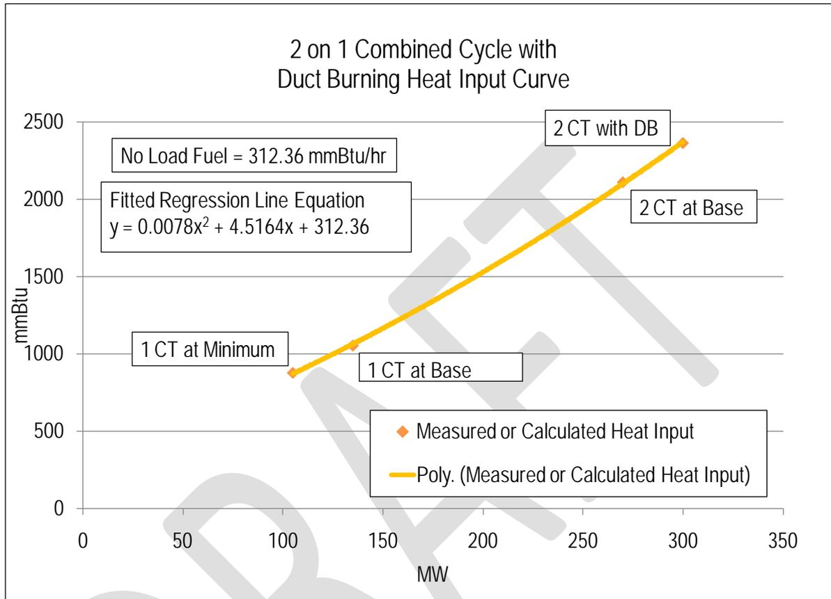
Each diamond in the graph above is a design heat input data point obtained from the original equipment manufacturer or calculated by heat balance. A regression analysis was performed on the design data to obtain the unit's Heat Input curve as a function of Output with natural gas as a fuel:
