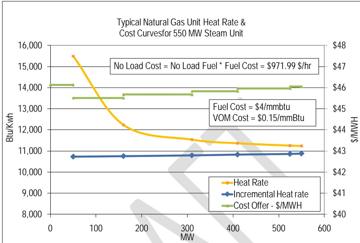
The No-Load cost was then raised to \$1007.76 until the first increment of the cost offer was less than \$1/MWh below the second increment, producing a monotonically increasing curve in the graph below:
