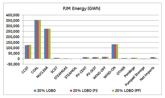
Figure 2-3: PJM Generation by Type in 20% LOBO Scenario under Original Forecast, 20% Forecast Improvement, and Perfect Forecast
