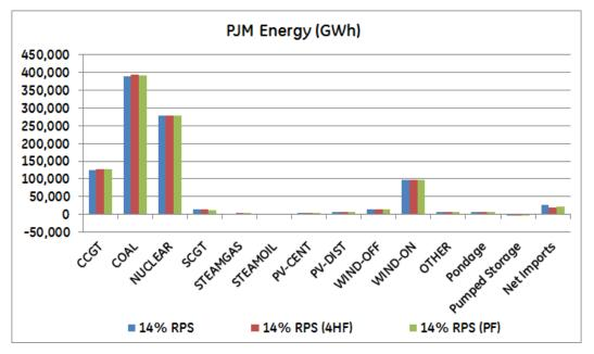
Figure 2-1: PJM Generation by Type in 14% RPS Scenario under Original Forecast, 4-Hour Forecast, and Perfect Forecast
