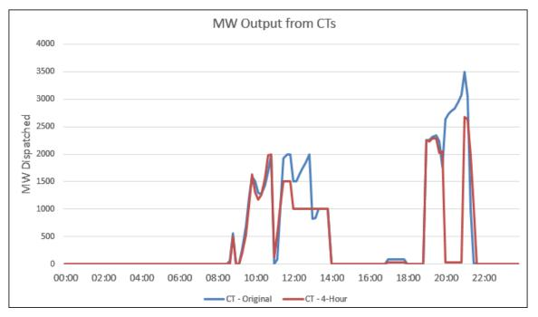
Figure 1-9: CT Dispatch by Interval (14% RPS - May 26)
