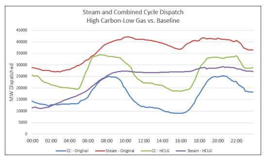
Figure 1-14: Steam/CC Dispatch by Interval (30% LOBO - February 17)
