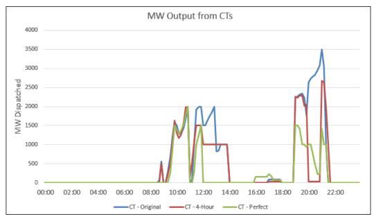
Figure 1-10: CT Dispatch by Interval (14% RPS - May 26)
