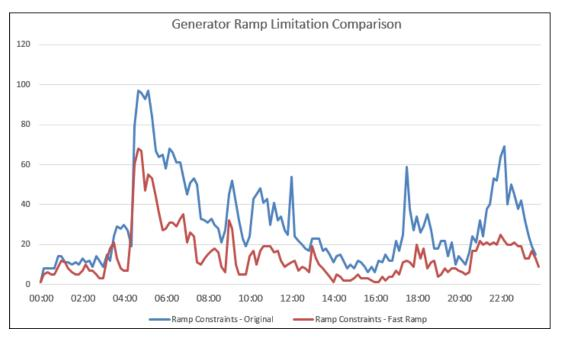
Figure 2-8: Number of Ramp Constrained Units with Existing Ramp Limits and 2%/min Ramp Limits
