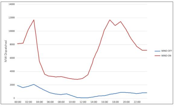
Figure 1-7: Wind Generation Output (14% RPS - May 26)
