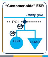
3. Metering and Method to Identify Direct Charging Energy at a Customer-side ESR
